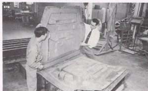
Matched temperature dies of epoxy resin
