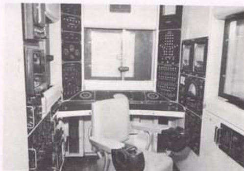
Typical mobile van for flight simulators built by GAC Console for training crewmen for ASW airship operation
