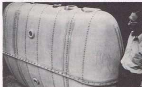
Airship fuel and ballast tank of cloth laminate
