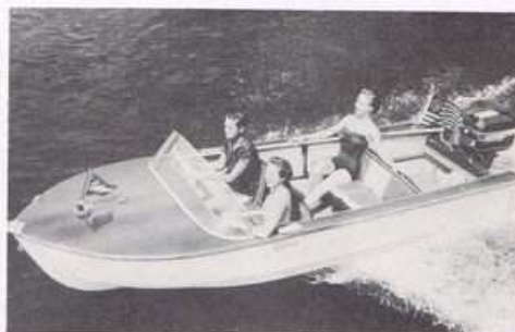
Boat hull made at GAC of fiberglass
