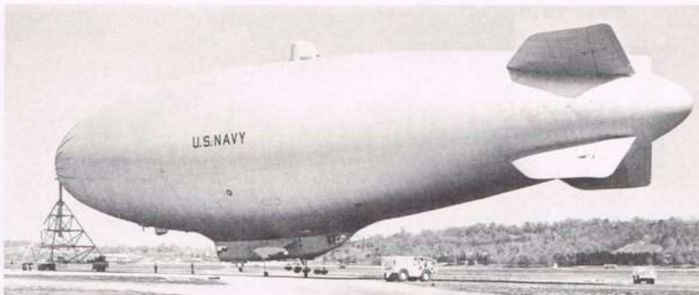
Like a missile, the airship is the heart around which is built a weapon system. The mooring mast and mechanical mule shown with this ZPG-3W airship form a part of the ground handling equipment, which has reduced manpower requirements to almost zero
