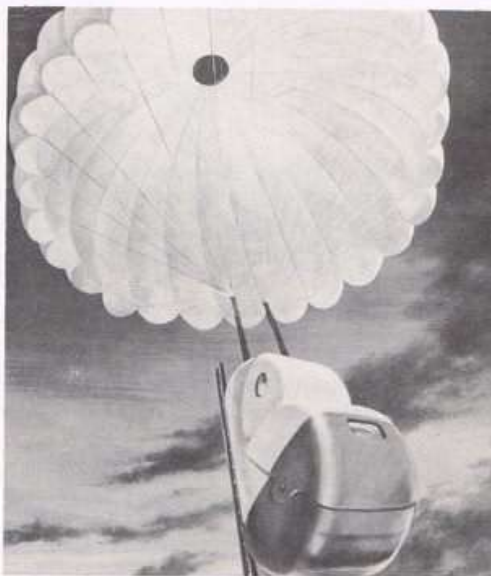
Artist shows how pilot would return safely to earth in GAC capsule after ejection at high altitude
