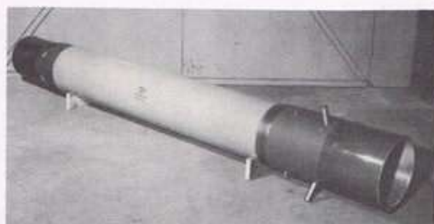
Two examples of the use of fiberglass at GAC — rocket motor cases (braided at top, reinforced at bottom)
